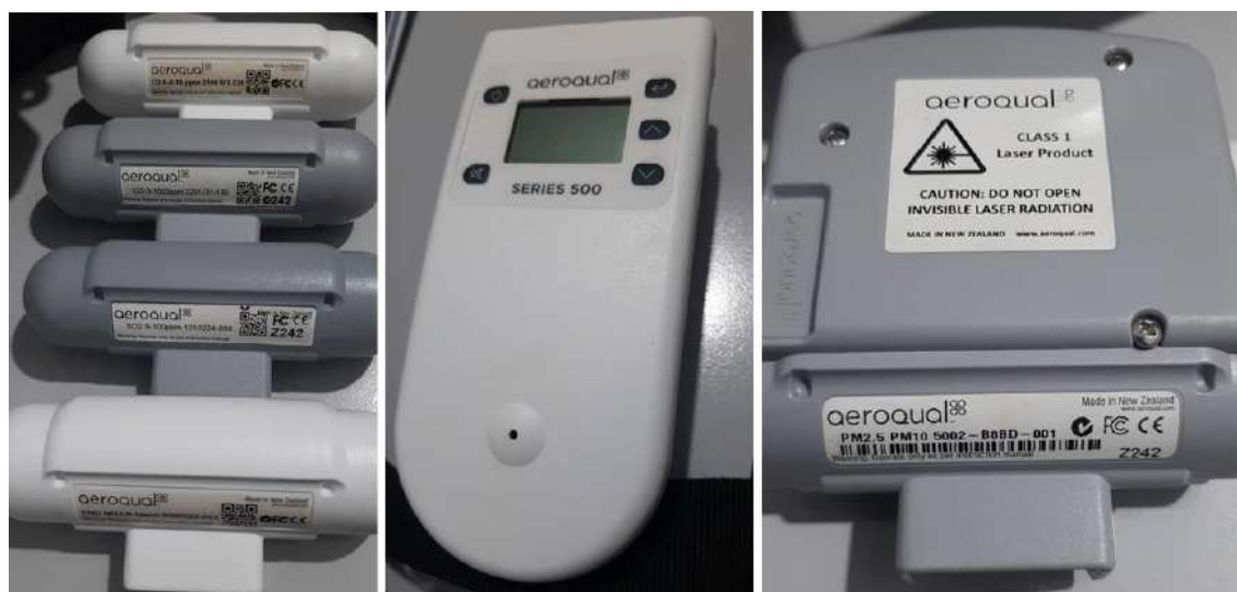
Photo 5-4: Air quality equipment (Aeroqual S500 and sensors for various pollutants)
