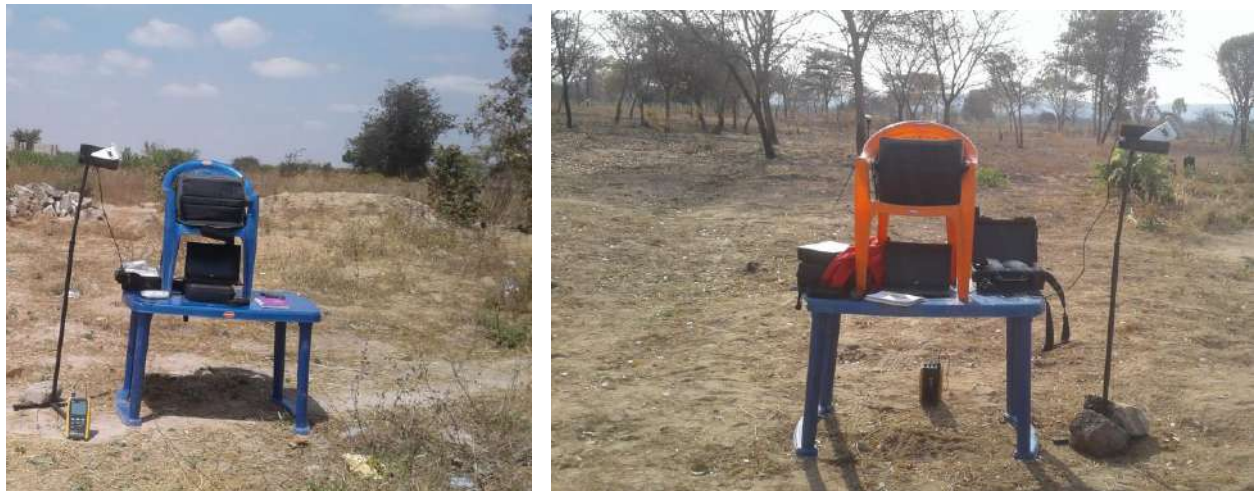
Photo 5-1: Vibration meter Lutron BVB-8207SD and monitoring set-up
